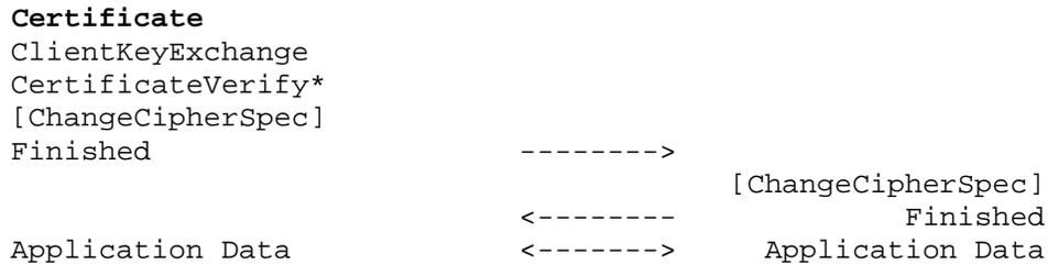
Fig. 1 - Message flow for a full handshake (RFC 2246)
